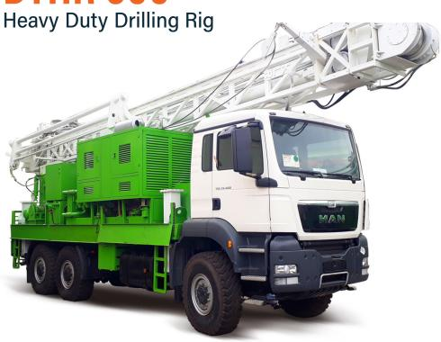
DTHR 600 is Top Head Drive DTH Cum Rotary Drilling Rig is capable of drilling in different formations such as Hard Rock by DTH, Un consolidated / Alluvial formations using Air/Water/Foam flush by Rotary Method up to a depth of 600 Meters, Under favorable drilling conditions.
